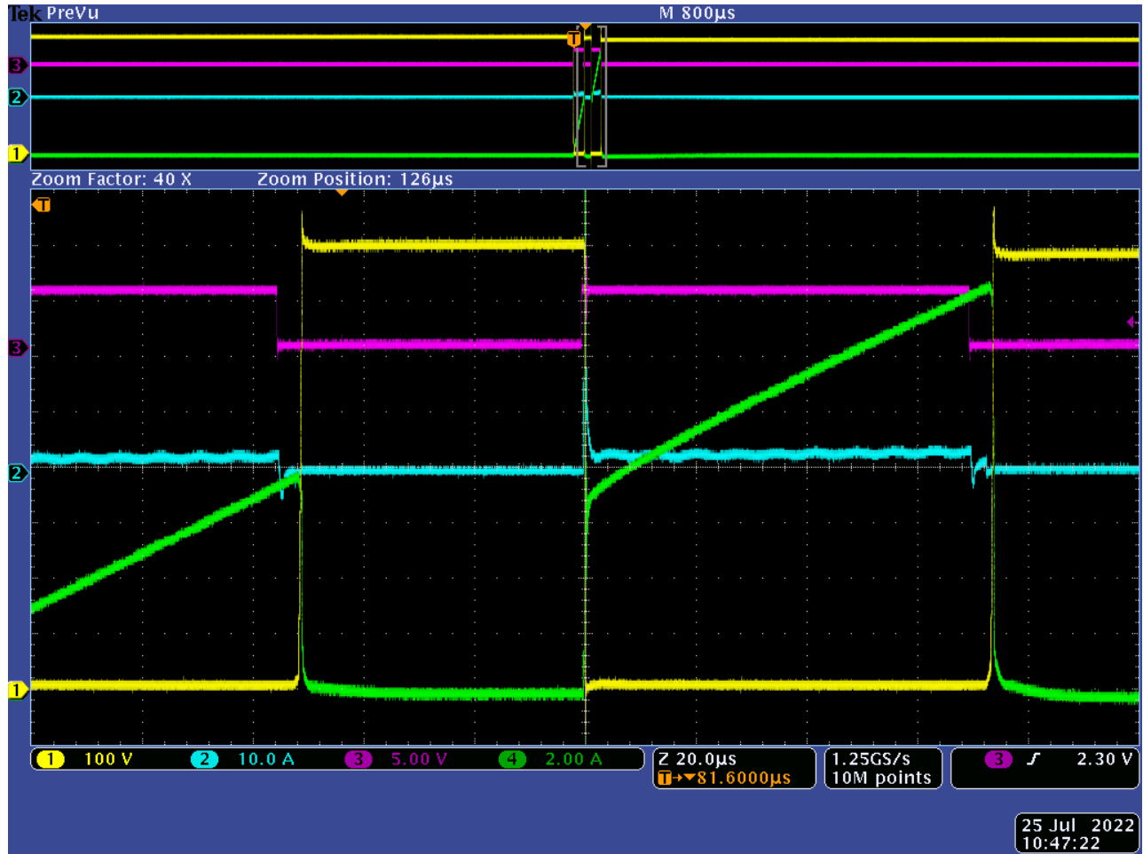
Figure 3: B-TRAN™ DPT waveforms
