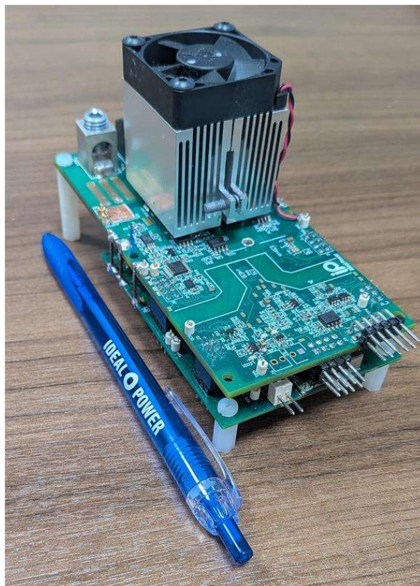
Figure 1: B-TRAN®-based SSCB evaluation board
