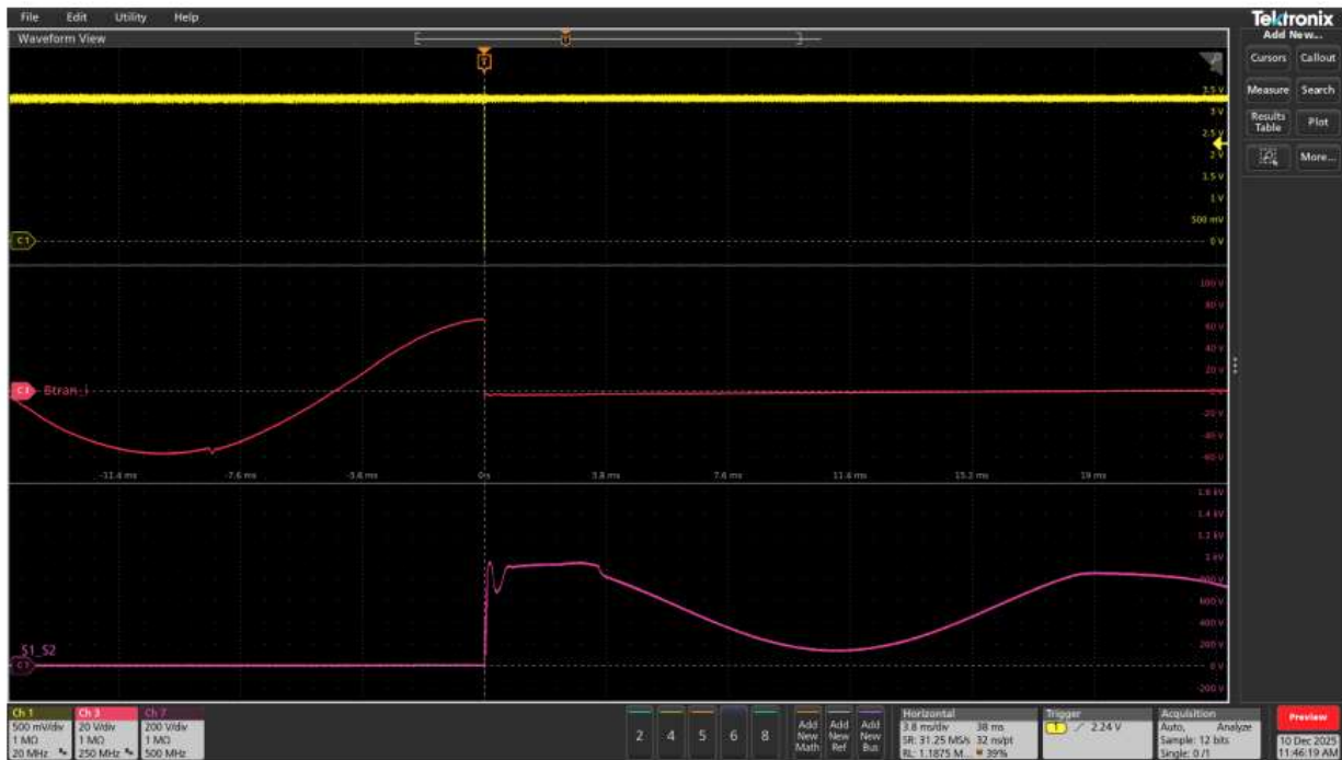
Figure 4: Example timing diagram showing AC tripping event at 300Vrms and 50A
